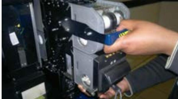
Removing the chassis from the housing.
